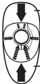
uneven force distribution into the seat tube. This can lead to function restrictions for dropper posts.
