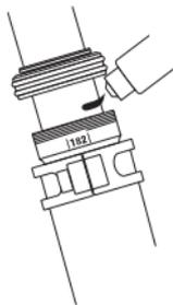
**7.5** Slide back the seal housing and tighten it by hand.
